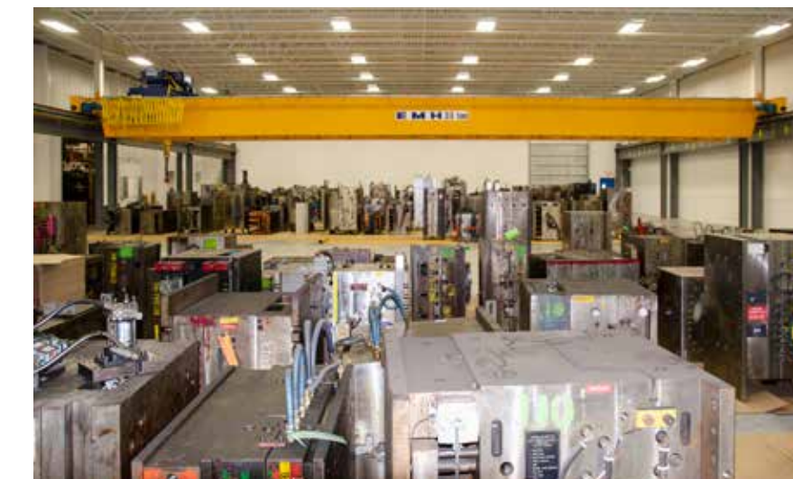
Interior of the new tool storage room with the overhead crane for moving large molds, December 2012.
