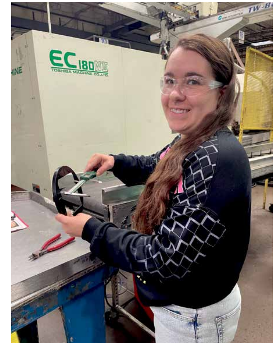
Quality inspector Marissa Lundberg uses a caliper to measure a part press-side. For more sophisticated measurements, the parts are taken from the press to the quality lab.
