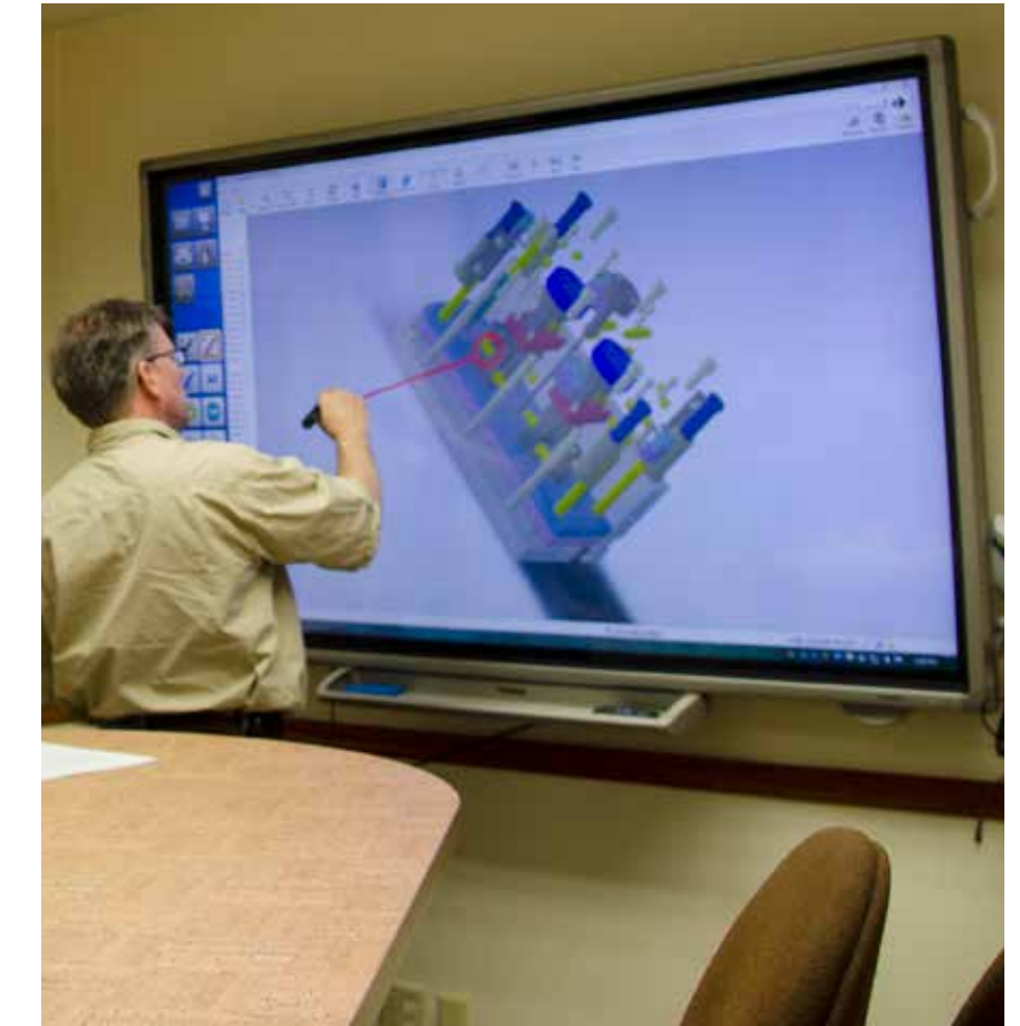
The engineering department installed an interactive whiteboard in 2013. The whiteboard can be connected to a computer to display images and data which the operator can mark up and highlight for demonstrations and conferencing.
