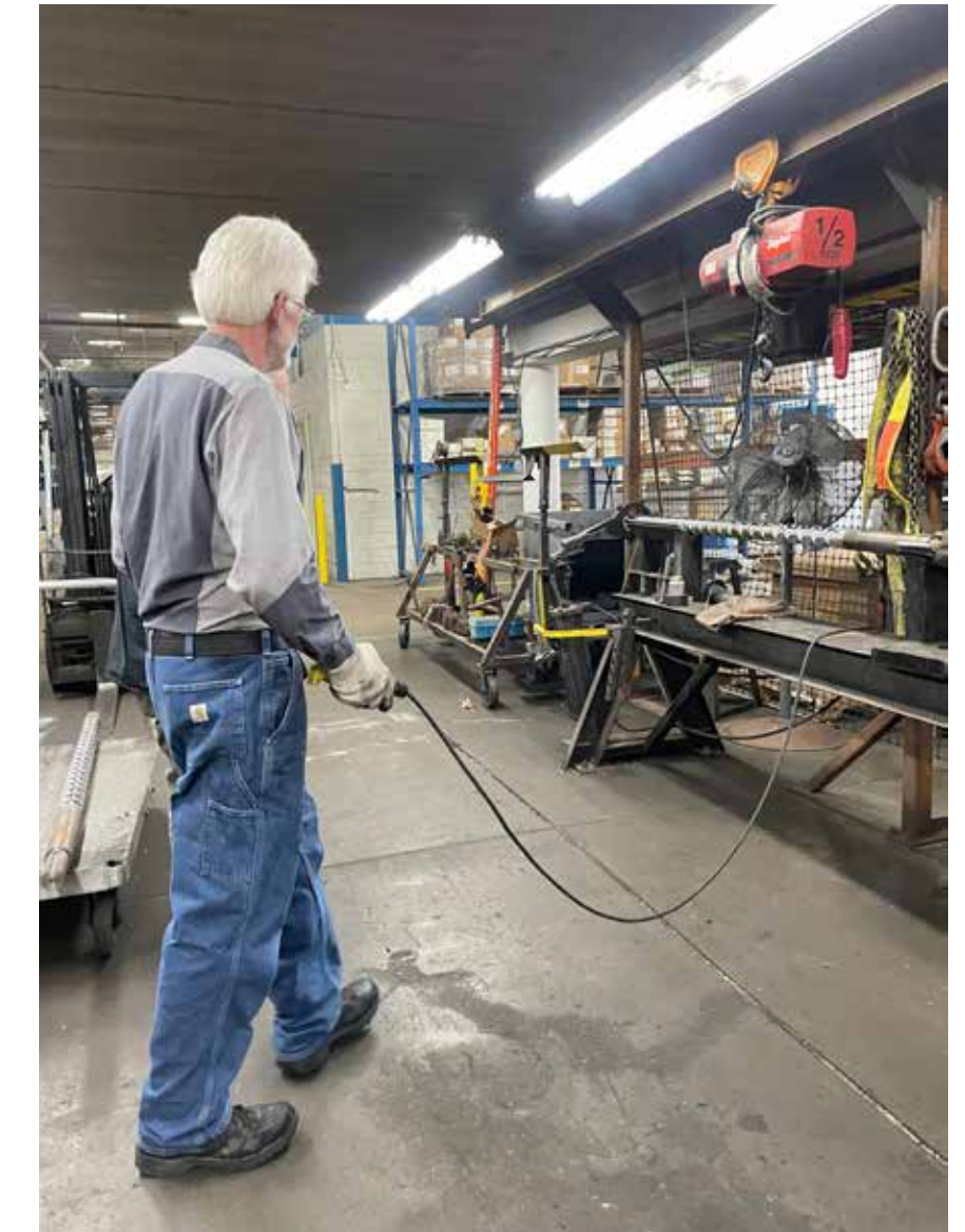
A large vice attaches to the screw tip and is turned by a hydraulic hoist to remove the tip from the screw.
