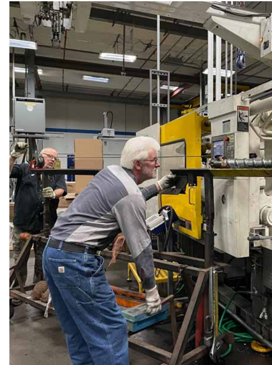
Maintenance technicians Robert Palmer (left) and Keith Voigt pulling a screw from a hot press and loading it onto the transportable cradle.
