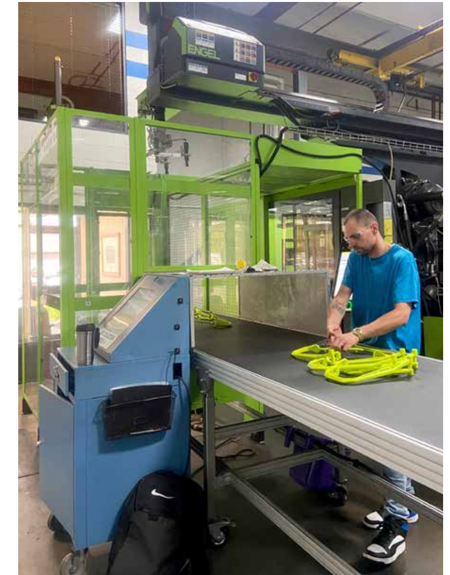
The 500-ton Engel, with its integrated linear robot, is one of the newer, high-efficiency molding machines.
