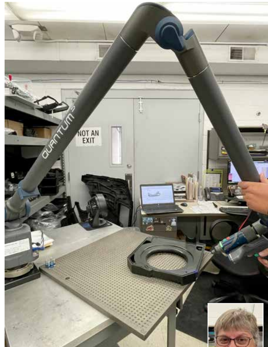
Layout tech Sue Schweigert (right) operating the FaroArm, a laser device that takes precise 3D measurements from multiple angles. Chelsea Nelson also operates the FaroArm.
