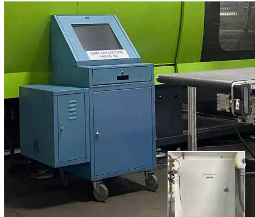
Blue cabinets at every press house a computer running IQMS ShopData that the operator uses to page for assistance and report rejects.
