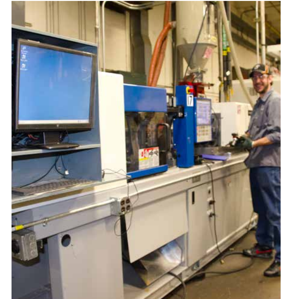
Process technician Adam Vohs setting up a brand-new, all-electric, 450-ton Toyo press in 2012.
