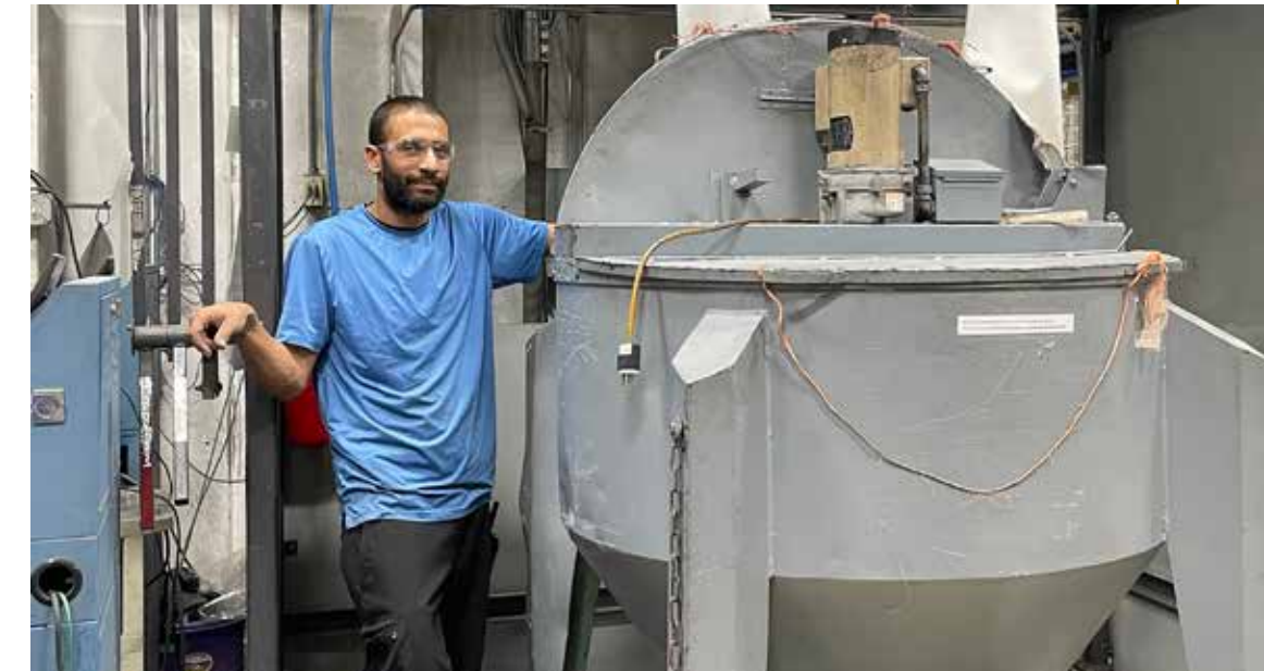
Material coordinator assistant Chris Trudeau running the hurricane mixer. This machine adds colorant or additives to the resin, which is fed into it directly from the silos. It takes about twenty minutes to mix a batch.
