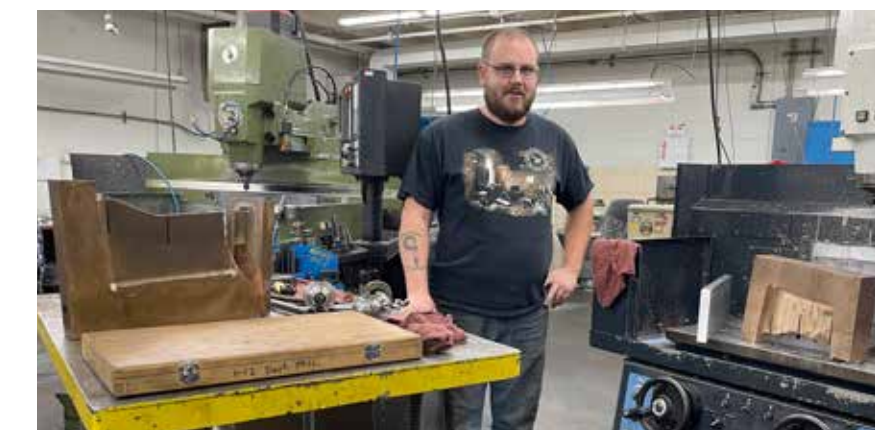
Journeyman toolmaker Sam Nelson rebuilding a mold for a livestock feeder. The broken tool is on the left and the new tool on the right.
